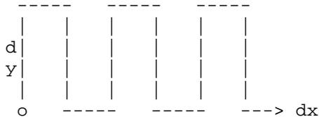
The scan starts at the point  $o$ , as specified with the commands below, and continues in the  $x$  and  $y$  directions in the range as specified with the commands below. At the end of the range, the motors are returned to the starting position and the scan is repeated.
